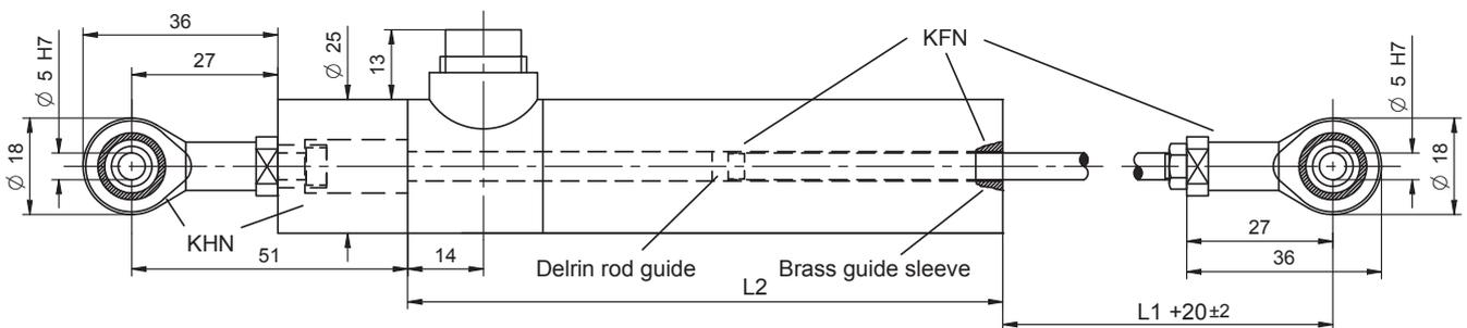
Inductive Linear Displacement Transducers Model IW 260
