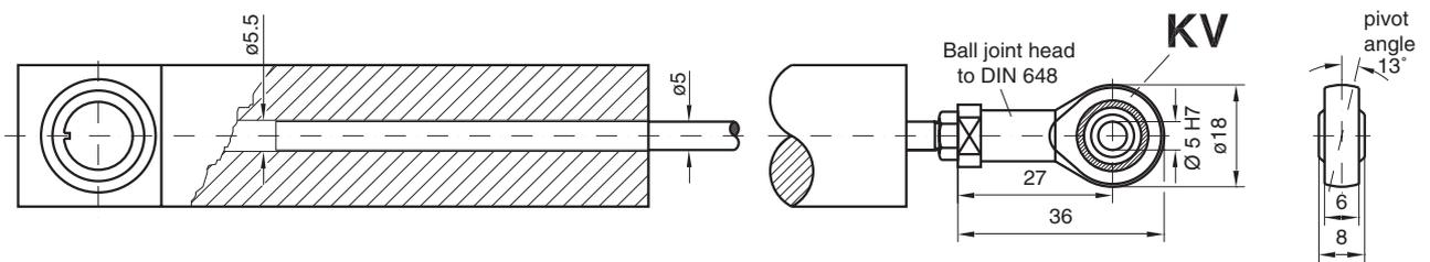
**Version with ball joints on plunger (KFN) and on end of case (KFH) (with rod guide, captivated)**
