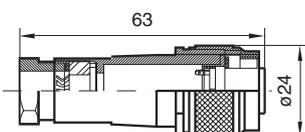
Metal case with outer ring connected to ground (must be ordered separately). BI 723M 3PS or 4PS (IP 66)
